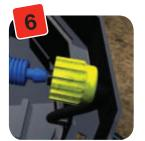
The AQUAvalve can now be connected to the 6mm pipe. Unscrew the yellow collar and push the pipe through it. Push the 6mm pipe on to the nozzle of the AQUAvalve and then replace the yellow collar by screwing it onto the AQUAvalve.
